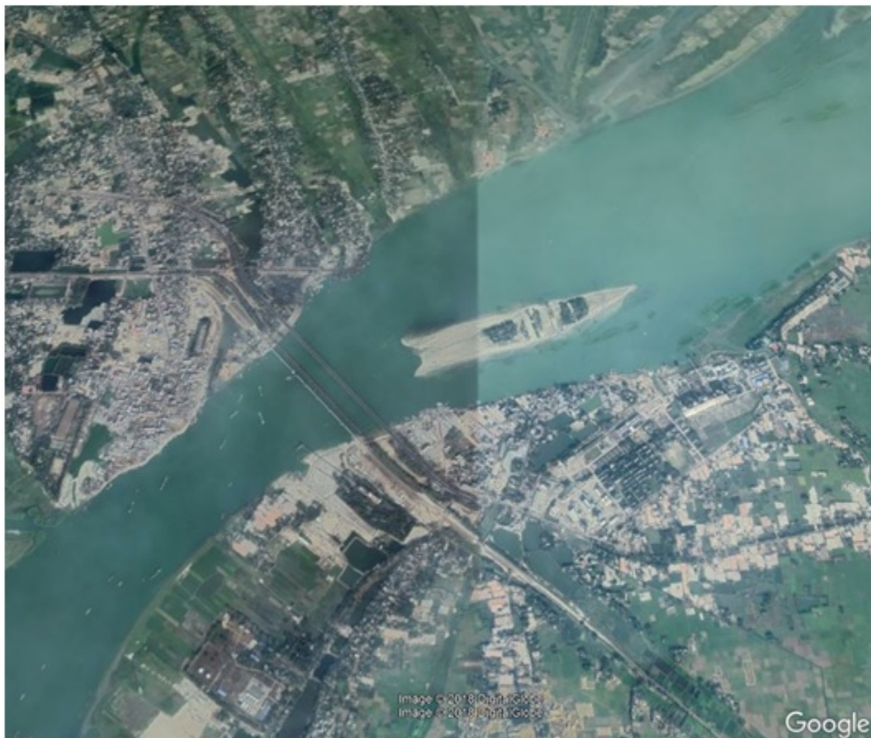
Figure 7: Google image showing the Bhairab Bridge on Meghna River and surrounding areas. Note the reduction in width of the river at Bhairab Bridge and widening of the river at upstream location near Kalipur (northeast corner of the image)
